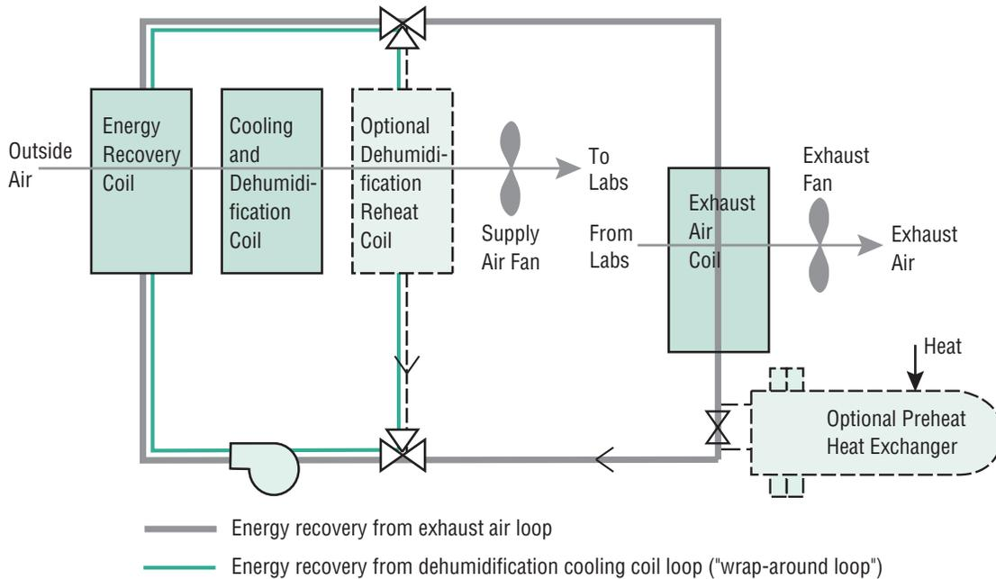
Figure 3. Run-around energy recovery loop with dehumidification
